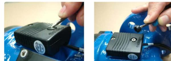
2. Remove seal cover from the screw using tool with sharp edge.
