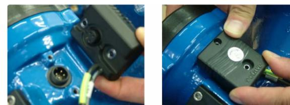
8. Tight both screws by hand only, using Allen key 3 mm to achieve symmetric o-ring pressure, **then apply the torque 2 N\*m with torque wrench.**
